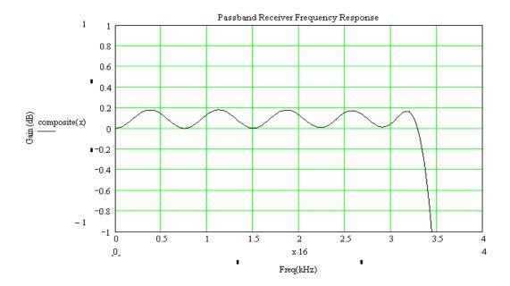
Figure 29: Pass-band Response of the Overall Receive Path
