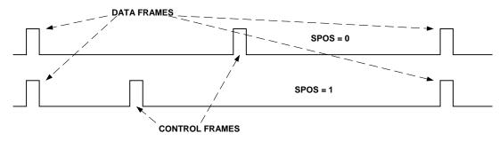
Figure 19: Control Frame Position versus SPOS
