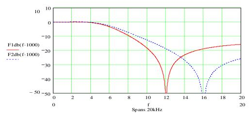
Figure 35: Magnitude Response of Billing Tone Notch Filter
