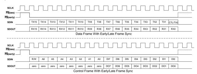
Figure 17: Serial Port Timing Diagram
