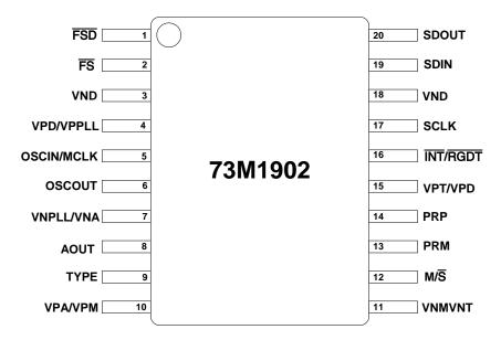
Figure 2: 73M1902 20-Pin TSSOP Pinout
