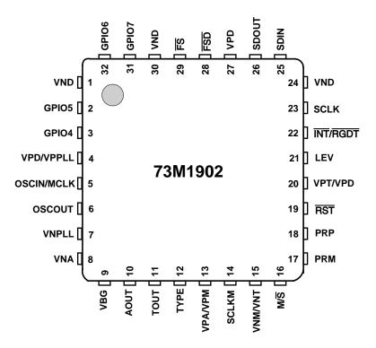
Figure 4: 73M1902 32-Pin QFN Pinout
