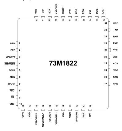
Figure 6: 73M1822 42-Pin Pinout
