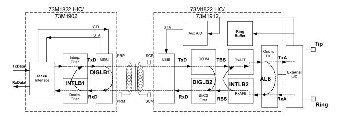
Figure 36: Loopback Modes Highlighted
