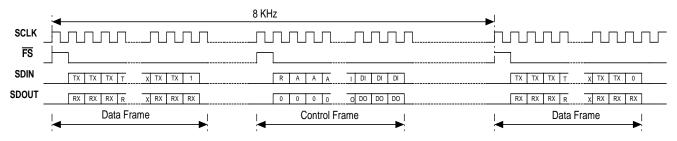
Figure 18: Data and Control Frames Timing Diagram
