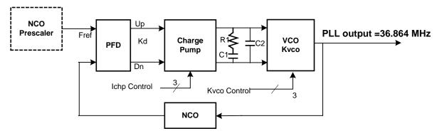
Figure 16: PLL Block Diagram
