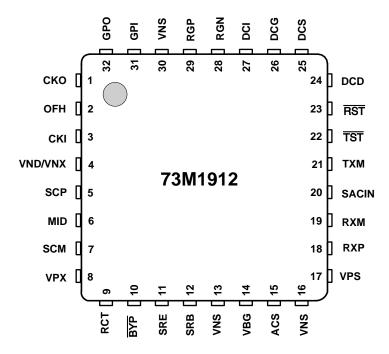
Figure 5: 73M1912 32-Pin QFN Pinout
