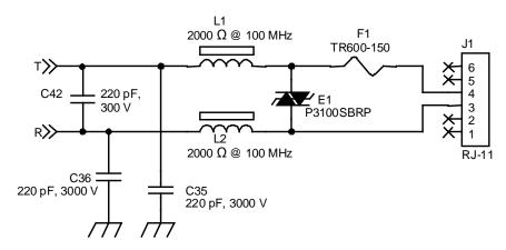
Figure 12: Suggested Over-voltage Protection and EMI Suppression Circuit
