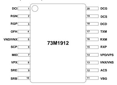
Figure 3: 73M1912 20-Pin TSSOP Pinout
