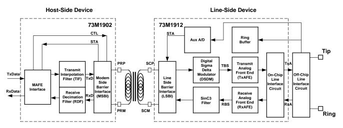
Figure 1: Simple 73M1x22 Reference Block Diagram
