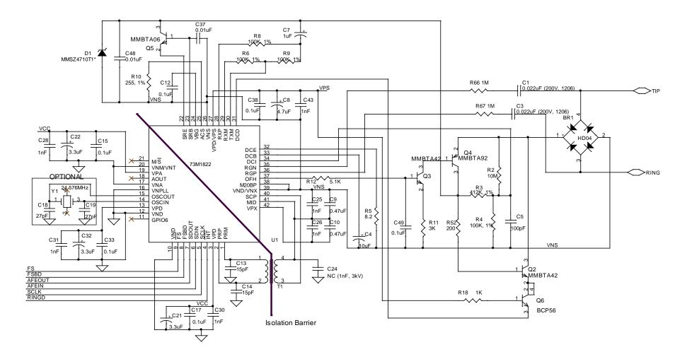
Figure 11: Recommended Circuit for the 73M1822
