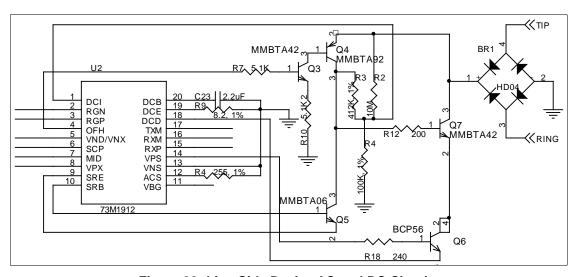
Figure 30: Line-Side Device AC and DC Circuits
