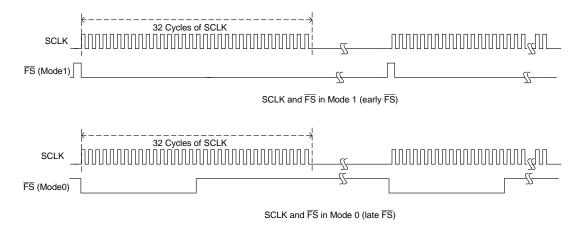
Figure 20: SCLK and  $\overline{FS}$  with SCKM = 0
