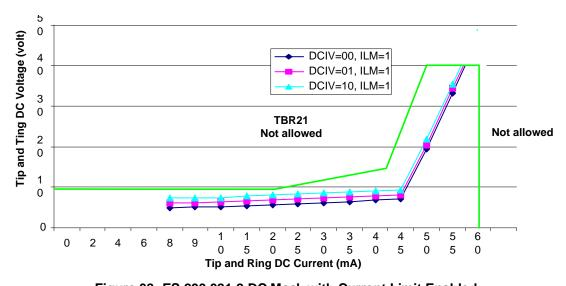
Figure 38: ES 203 021-2 DC Mask with Current Limit Enabled
