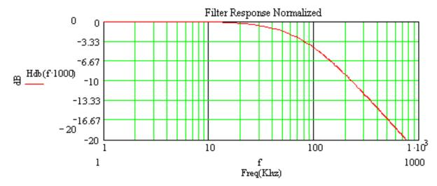
Figure 8: Call Progress Monitor Frequency Response
