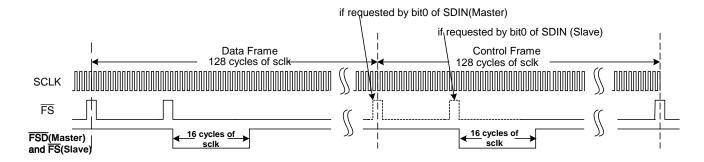
Figure 22: Master/Slave Serial Timing Diagram
