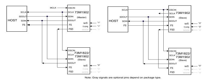
Figure 21: Example Connections for Master and Slave Operation
