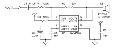
Figure 9: Demo Board Circuit Connecting AOUT to a Speaker
