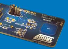
Atmel EVK1012A Evaluation board for the Atmel AT42QT1012 controller
