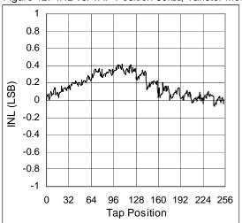
Figure 14. INL vs. TAP Position 100k $\Omega$ , Varistor
