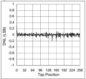
Figure 13. DNL vs. TAP Position 100 $k\Omega$ , Varistor Mode Mode
