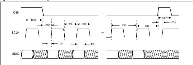
Figure 20. Serial Data Timing
