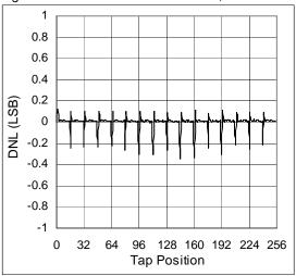
Figure 5. DNL vs. TAP Position  $50k\Omega$ , Divider Mode
