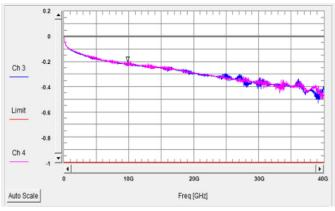
Fig. 2: Low insertion loss of 2.92 mm female to 2.92 mm female adapter
