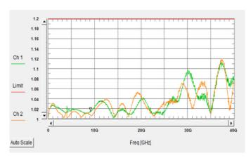
Fig.1: VSWR performance of 2.92 mm female to 2.92 mm female adapter
