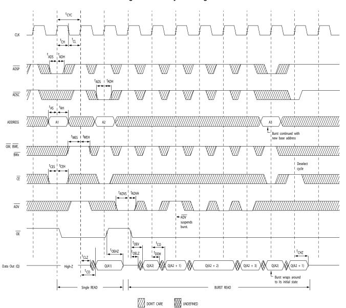
Figure 6. Read Cycle Timing <sup>[26]</sup>
