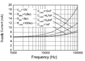
Supply Current vs Capacitive Load
