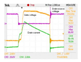
Fig 1a: Continuous Conduction Mode (CCM)
