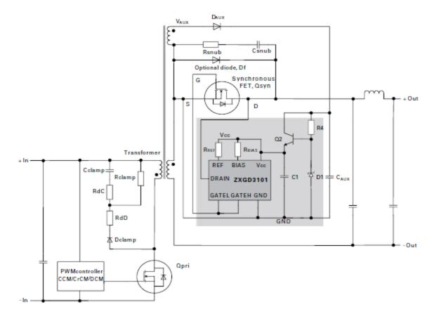
Figure 3 - Example connection for high side synchronous rectification
