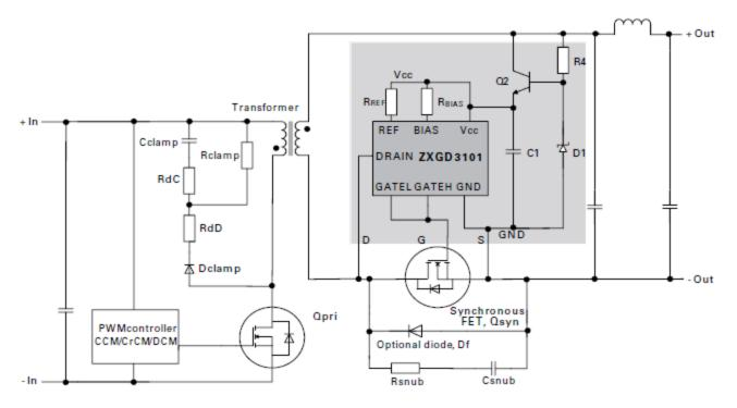
Figure 2 - Example connection for low side synchronous rectification
