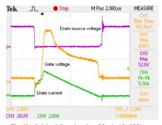
Fig 1b: Critical Conduction Mode (CrCM)
