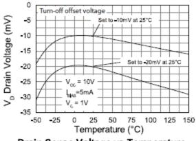
Drain Sense Voltage vs Temperature
