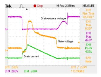
Fig 1c: Discontinuous Conduction Mode (DCM)
