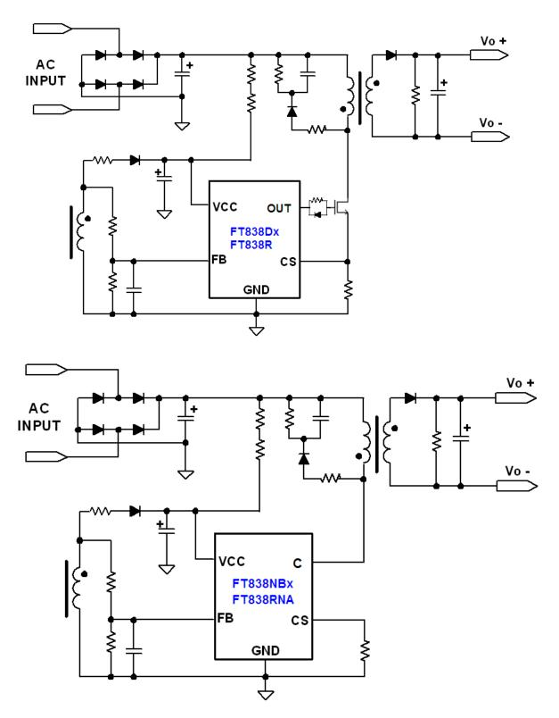
Figure 1: FT838xx Typical Application Circuit
