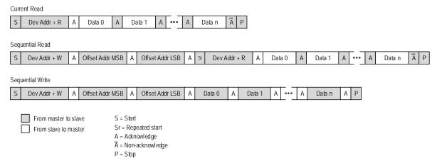
Figure 6. I<sup>2</sup>C Slave Read and Write Cycle Sequencing
