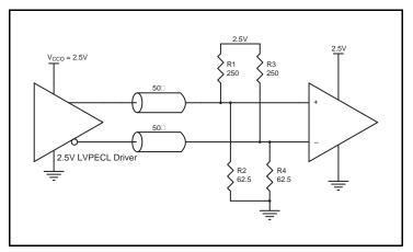
Figure 14A. 2.5V LVPECL Driver Termination Example
