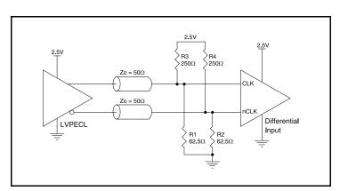
Figure 11B. CLKx/nCLKx Input Driven by a 2.5V LVPECL Driver
