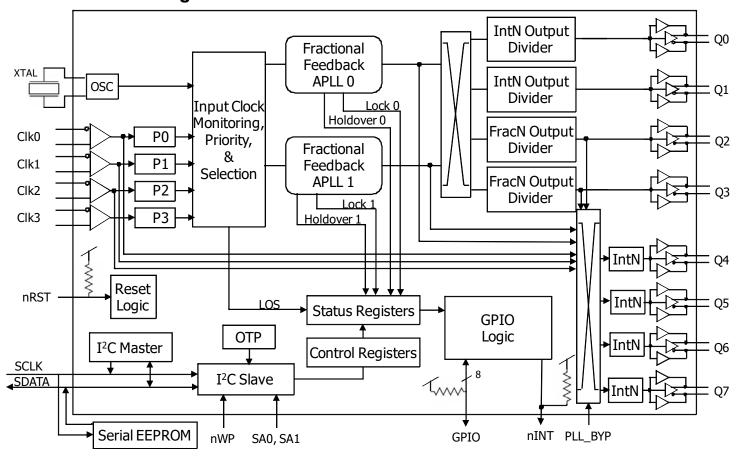
Figure 1. 8T49N282 Functional Block Diagram
