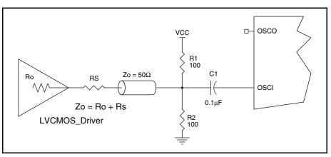
Figure 8A. General Diagram for LVCMOS Driver to XTAL Input Interface
