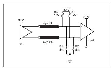
Figure 13B. 3.3V LVPECL Output Termination
