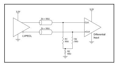
Figure 10D. CLKx/nCLKx Input Driven by a 3.3V LVPECL Driver
