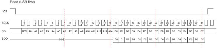
Figure 3. SPI Read Sequencing Diagram
