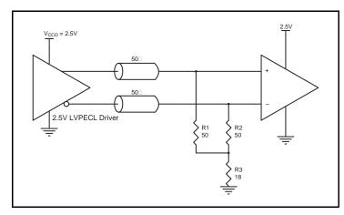
Figure 14C. 2.5V LVPECL Driver Termination Example
