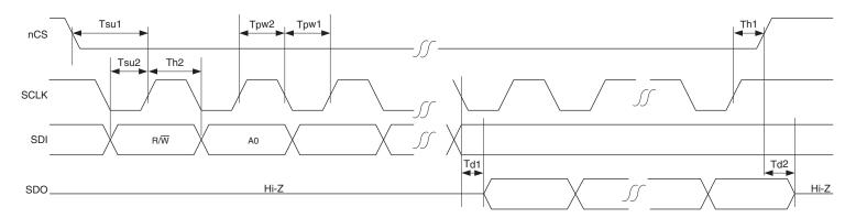
Figure 5. SPI Read/Write Timing Diagram
