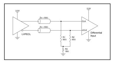
Figure 11C. CLKx/nCLKx Input Driven by a 2.5V LVPECL Driver
