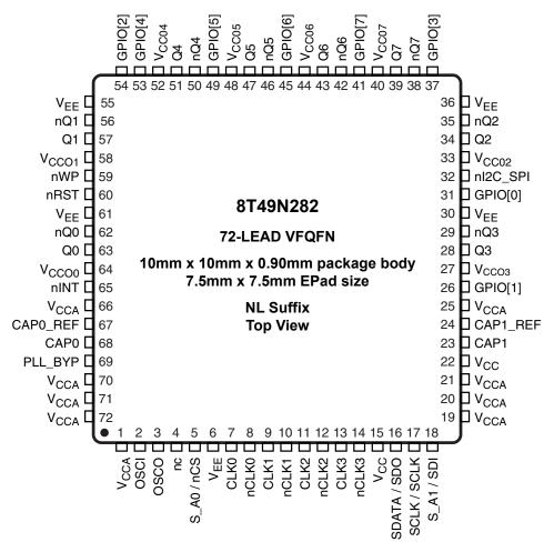
Figure 2. Pinout Drawing
