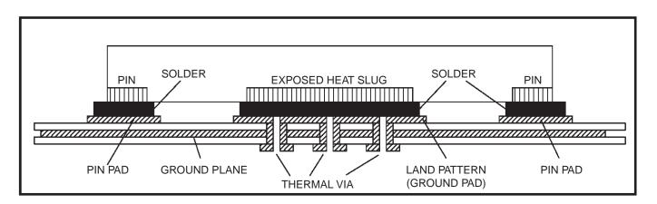
Figure 15. P.C. Assembly for Exposed Pad Thermal Release Path – Side View (drawing not to scale)
