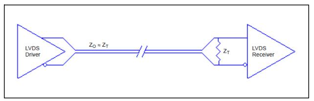
Figure 12A. Standard LVDS Termination
