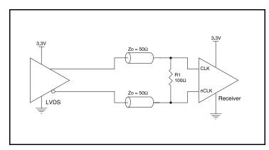
Figure 10E. CLKx/nCLKx Input Driven by a 3.3V LVDS Driver
