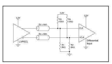
Figure 10B. CLKx/nCLKx Input Driven by a 3.3V LVPECL Driver
