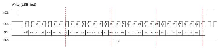
Figure 4. SPI Write Sequencing Diagram
