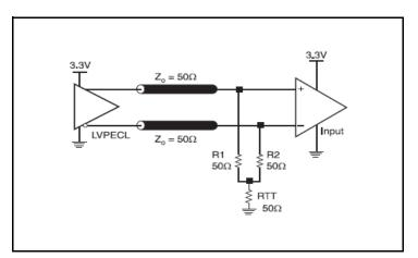
Figure 13A. 3.3V LVPECL Output Termination
