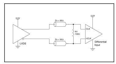
Figure 11D. CLKx/nCLKx Input Driven by a 2.5V LVDS Driver
