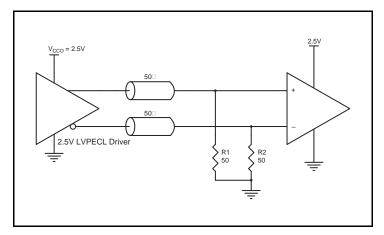
Figure 14B. 2.5V LVPECL Driver Termination Example
