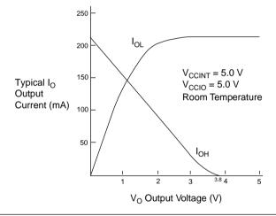
Figure 6. Output Drive Characteristics of MAX 5000 Devices
