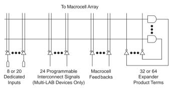
Expanders are fed by all signals in the LAB. One expander can feed all macrocells in the LAB or multiple product terms in the same macrocell. Because expanders also feed the secondary product terms of each macrocell, complex logic functions can be implemented without using additional macrocells. A small delay (t<sub>SEXP</sub>) is incurred when shared expanders are used.
