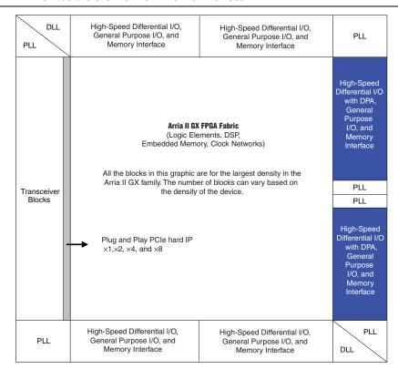
Figure 1-1. Architecture Overview for Arria II GX Devices
