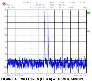
CLOCK, 500kHz SPACING (67dBc - 10MHz WINDOW, 6dB PAD)
