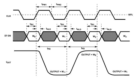
FIGURE 8. PROPAGATION DELAY, SETUP TIME, HOLD TIME AND MINIMUM PULSE WIDTH DIAGRAM
