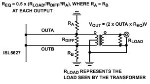
FIGURE 7. ALTERNATIVE OUTPUT LOADING
