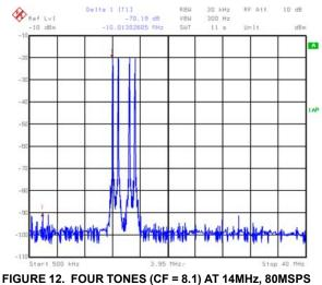
IGURE 12. FOUR TONES (CF = 8.1) AT 14MHz, 80MSPS CLOCK, 800kHz SPACING (70dBc - NYQUIST, 6dB PAD)
