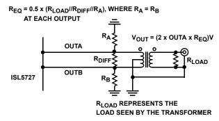
FIGURE 14. ALTERNATIVE OUTPUT LOADING
