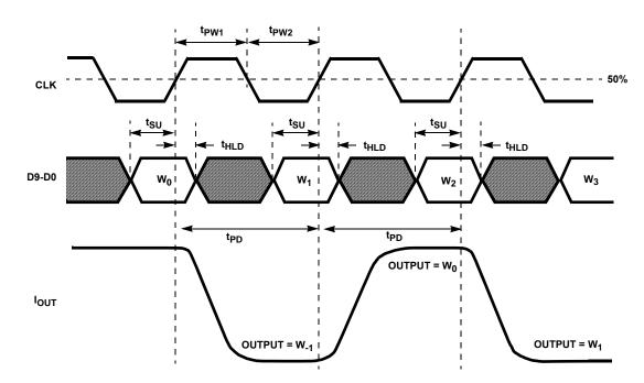
FIGURE 15. PROPAGATION DELAY, SETUP TIME, HOLD TIME AND MINIMUM PULSE WIDTH DIAGRAM
