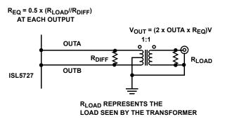
FIGURE 13. OUTPUT LOADING FOR DATASHEET MEASUREMENTS
