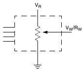
Three terminal Potentiometer; Variable voltage divider
