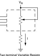
Two terminal Variable Resistor; Variable current
