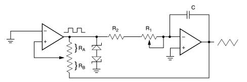
frequency  $\propto R_1,\,R_2,\,C$  amplitude  $\propto R_A,\,R_B$
