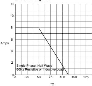
Average Forward Rectified Current - Amperes/ersus Ambient Temperature -°C
