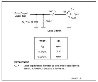
$t_{PLZ}$  and  $t_{PHZ}$  are the same as  $t_{dis}$ .  $t_{PZL}$  and  $t_{PZH}$  are the same as  $t_{en}$ .
