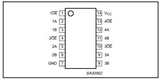
Figure 1. SO14, SSOP14, and TSSOP14
