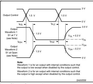
$t_{\mbox{\scriptsize PLZ}}$  and  $t_{\mbox{\scriptsize PHZ}}$  are the same as  $t_{\mbox{\scriptsize dis}}.$
