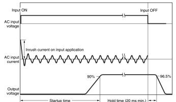
Note: A maximum startup time of 1,000 ms is required. Construct a system configuration that considers the startup time of other devices.
