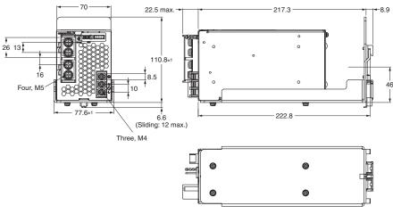
Note: Use a metal DIN Rail when mounting a 300-W model to a DIN Rail.
