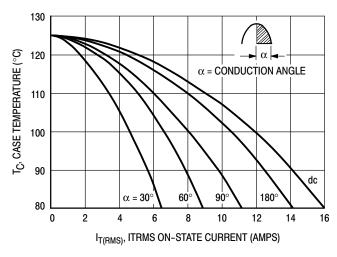
Figure 1. Typical RMS Current Derating
