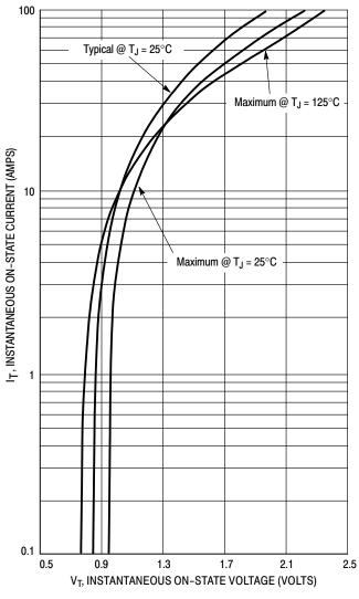
Figure 3. Typical On-State Characteristics
