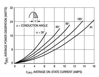
Figure 2. On State Power Dissipation
