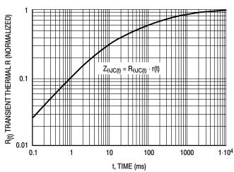
**Figure 4. Transient Thermal Response**
