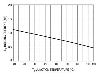
Figure 7. Typical Holding Current versus Junction Temperature
