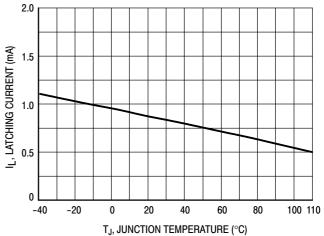
Figure 8. Typical Latching Current versus Junction Temperature
