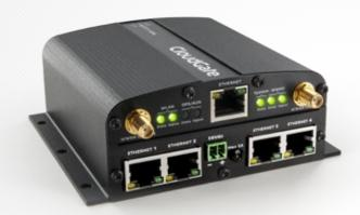
The Ethernet switch allows more than on device to be connected to CloudGate Intelligent M2M Gateway. It supports IEEE 802.3 flow control for Full Duplex mode and backpressure for half-duplex mode and supports MAC address auto-learning and auto-aging.
