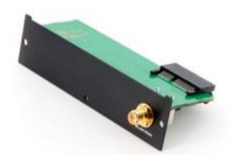
The Monnit® expansion card inserts into the front or rear expansion slot of the CloudGate and allows the CloudGate to function as a gateway for wireless Monnit® devices like sensors and relays over the 433MHz, the 868MHz or the 900MHz band. Monnit® Wifi sensors are not supported.
