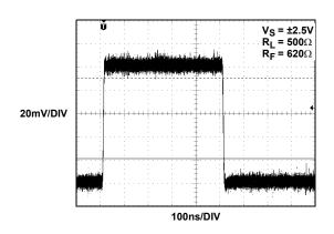
FIGURE 35. SMALL SIGNAL STEP RESPONSE
