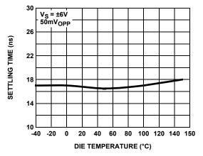
FIGURE 39. 0.1% SETTLING TIME vs TEMPERATURE
