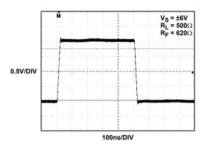
FIGURE 32. LARGE SIGNAL STEP RESPONSE
