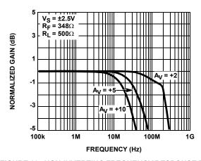
FIGURE 16. NON-INVERTING FREQUENCY RESPONSE FOR VARIOUS A<sub>V</sub>
