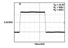
FIGURE 33. LARGE SIGNAL STEP RESPONSE
