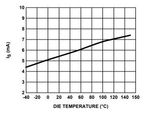
FIGURE 36. SUPPLY CURRENT vs TEMPERATURE
