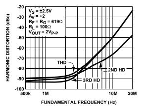
FIGURE 22. HARMONIC DISTORTION vs FREQUENCY
