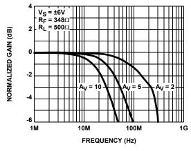
FIGURE 2. NON-INVERTING FREQUENCY RESPONSE (GAIN)
