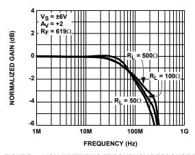
FIGURE 4. NON-INVERTING FREQUENCY RESPONSE FOR VARIOUS  $R_{\rm L}$
