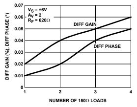
FIGURE 31. DIFFERENTIAL GAIN/PHASE
