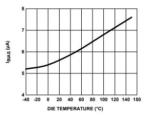
FIGURE 41.  $I_{\mbox{\footnotesize BIAS}}$  CURRENT vs TEMPERATURE
