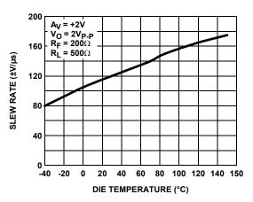
FIGURE 38. SLEW RATE vs TEMPERATURE
