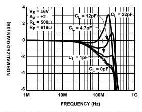
FIGURE 3. NON-INVERTING FREQUENCY RESPONSE FOR VARIOUS  $C_L$
