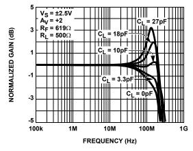
FIGURE 17. NON-INVERTING FREQUENCY RESPONSE FOR VARIOUS  $C_L$
