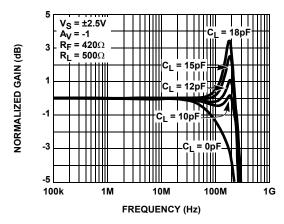
FIGURE 13. INVERTING FREQUENCY RESPONSE FOR VARIOUS C<sub>I</sub>
