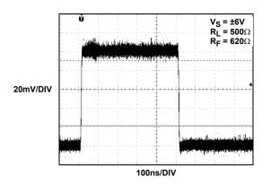
FIGURE 34. SMALL SIGNAL STEP RESPONSE
