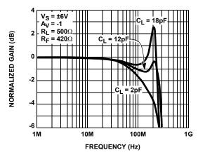
FIGURE 8. INVERTING FREQUENCY RESPONSE FOR VARIOUS CI
