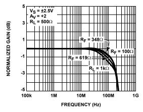
FIGURE 15. NON-INVERTING FREQUENCY RESPONSE FOR VARIOUS  $R_{\rm F}$
