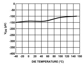
FIGURE 40.  $V_{OS}$  vs TEMPERATURE
