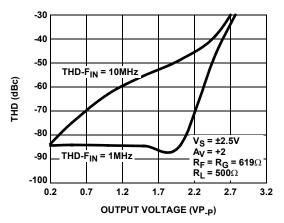
FIGURE 23. THD vs OUTPUT VOLTAGE
