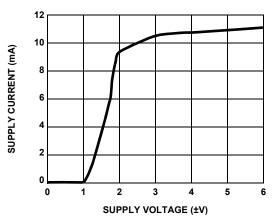
FIGURE 24. SUPPLY CURRENT vs SUPPLY VOLTAGE
