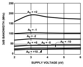
FIGURE 25. 3dB BANDWIDTH vs SUPPLY VOLTAGE
