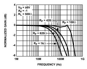
FIGURE 6. INVERTING FREQUENCY RESPONSE FOR VARIOUS  $R_{\rm F}$
