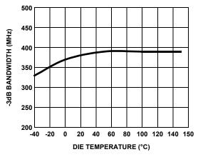
FIGURE 37. -3dB BANDWIDTH vs TEMPERATURE
