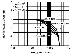
FIGURE 1. NON-INVERTING FREQUENCY RESPONSE FOR VARIOUS  $R_{\text{F}}$
