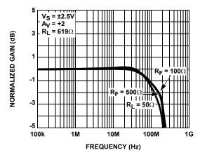
FIGURE 18. NON-INVERTING FREQUENCY RESPONSE FOR VARIOUS  $R_L$
