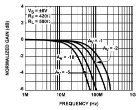
FIGURE 7. INVERTING FREQUENCY RESPONSE (GAIN)
