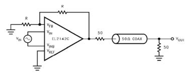
FIGURE 2. COAXIAL CABLE DRIVER PAIR APPLICATION
