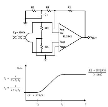
FIGURE 4. COMPENSATED LINE RECEIVER
