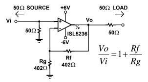
FIGURE 37. G = +2V/V CHARACTERIZATION CIRCUIT
