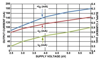
FIGURE 30. SUPPLY CURRENT vs SUPPLY VOLTAGE
