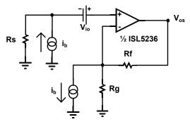
FIGURE 40. OUTPUT DC OFFSET ANALYSIS CIRCUIT
