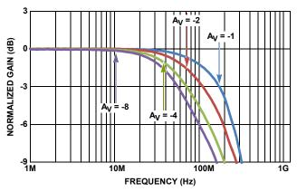
FIGURE 3. INVERTING SMALL SIGNAL FREQUENCY RESPONSE
