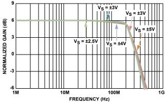
FIGURE 26. NON-INVERTING SMALL SIGNAL RESPONSE vs SUPPLY VOLTAGE
