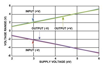
FIGURE 31. COMMON MODE INPUT RANGE AND OUTPUT SWING VS SUPPLY VOLTAGE
