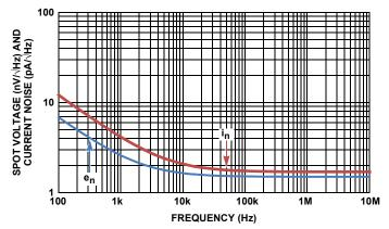
FIGURE 36. INPUT SPOT NOISE VOLTAGE AND CURRENT
