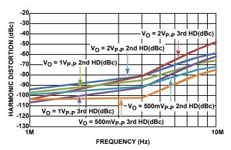
FIGURE 11. INVERTING HD2 AND HD3 vs OUTPUT  $V_{P\mbox{-}P}$
