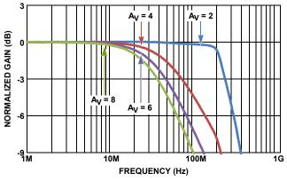
FIGURE 32. NON-INVERTING SMALL SIGNAL RESPONSE vs GAIN
