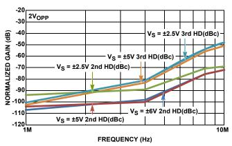
FIGURE 28. NON-INVERTING HD2 AND HD3 vs SUPPLY VOLTAGE
