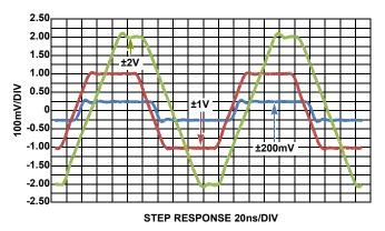
FIGURE 15. INVERTING LARGE AND SMALL SIGNAL STEP RESPONSE
