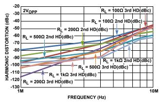
FIGURE 13. INVERTING HD2 AND HD3 vs R<sub>LOAD</sub>
