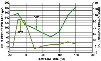
FIGURE 7. INPUT OFFSET VOLTAGE AND CURRENT vs TEMPERATURE
