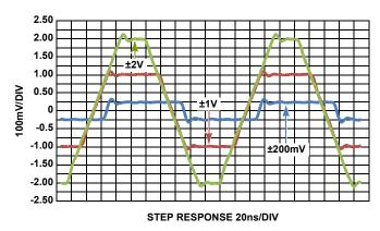
FIGURE 14. NON-INVERTING LARGE AND SMALL SIGNAL STEP RESPONSE
