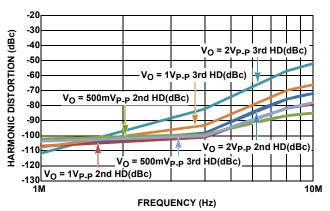
FIGURE 10. NON-INVERTING HD2 AND HD3 vs OUTPUT Vp.p
