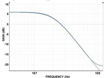
FIGURE 42. SIMULATED vs IDEAL FILTER RESPONSE COMPARISON
