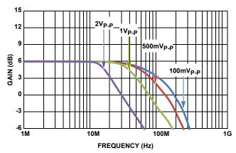
FIGURE 35. INVERTING LARGE SIGNAL RESPONSE
