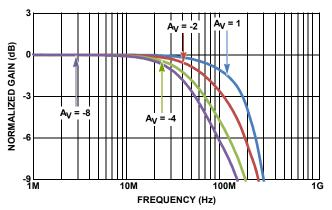
FIGURE 33. INVERTING SMALL SIGNAL RESPONSE vs GAIN
