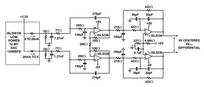
LOW POWER, LOW NOISE, DIFFERENTIAL DAC OUTPUT TRANSIMPEDANCE WITH A 5TH ORDER, 5MHz, BUTTERWORTH FILTER
