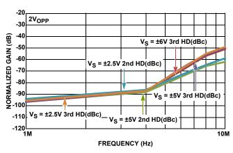
FIGURE 29. INVERTING HD2 AND HD3 vs SUPPLY VOLTAGE
