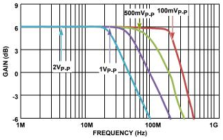
FIGURE 4. NON-INVERTING LARGE SIGNAL RESPONSE
