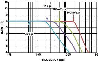
FIGURE 34. NON-INVERTING LARGE SIGNAL RESPONSE
