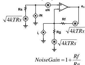
FIGURE 39. OP AMP NON-INVERTING NOISE ANALYSIS CIRCUIT
