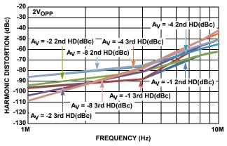
FIGURE 9. INVERTING HD2 AND HD3 vs GAIN
