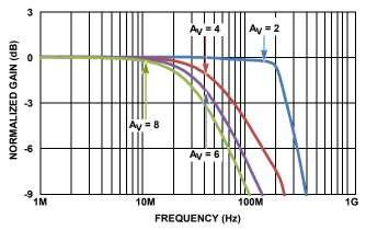
FIGURE 2. NON-INVERTING SMALL SIGNAL FREQUENCY **REPONSE vs GAIN**
