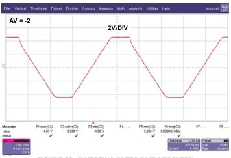
FIGURE 17. INVERTING OVERDRIVE RECOVERY
