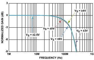
FIGURE 27. INVERTING SMALL SIGNAL RESPONSE VS SUPPLY VOLTAGE
