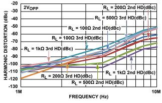
FIGURE 12. NON-INVERTING HD2 AND HD3 vs  $R_{LOAD}$
