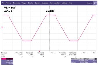
FIGURE 16. NON-INVERTING OVERDRIVE RECOVERY
