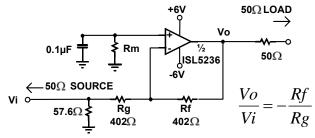
FIGURE 38. G = -1V/V CHARACTERIZATION CIRCUIT
