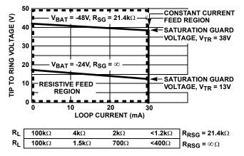
FIGURE 15. VTR vs IL AND RL
