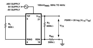
FIGURE 12. POWER SUPPLY REJECTION RATIO
