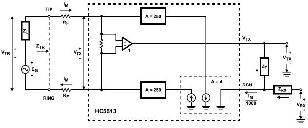
FIGURE 16. SIMPLIFIED AC TRANSMISSION CIRCUIT
