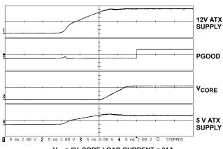
V<sub>IN</sub> = 5V, CORE LOAD CURRENT = 31A FREQUENCY 200kHz ATX SUPPLY ACTIVATED BY ATX "PS-ON PIN"
