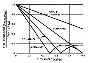
FIGURE 12. RIPPLE CURRENT vs DUTY CYCLE
