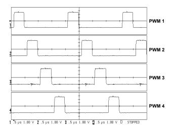
FIGURE 2. FOUR PHASE PWM OUTPUT AT 500kHz
