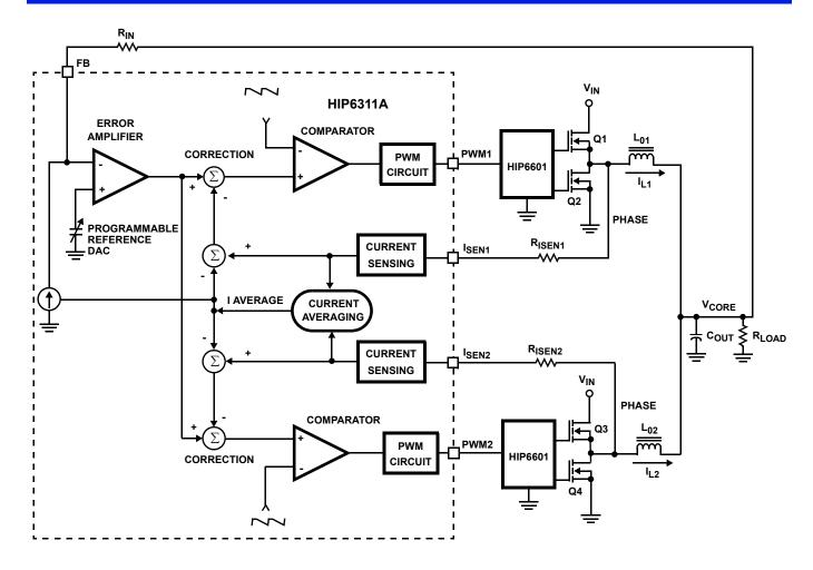
FIGURE 1. SIMPLIFIED BLOCK DIAGRAM OF THE HIP6311A VOLTAGE AND CURRENT CONTROL LOOPS FOR A TWO POWER CHANNEL REGULATOR
