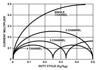
FIGURE 13. CURRENT MULTIPLIER vs DUTY CYCLE
