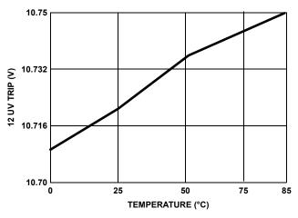
FIGURE 8. 12V UV Vth vs TEMPERATURE
