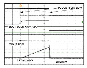
FIGURE 3. FLTN & PGOOD FUNCTIONAL WAVEFORM
