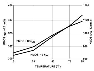
FIGURE 7. ron vs TEMPERATURE
