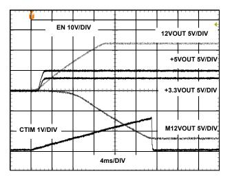
FIGURE 14. ISL6111 TURN-ON INTO NOMINAL LOAD
