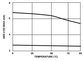
FIGURE 10. BIAS CURRENT vs TEMPERATURE
