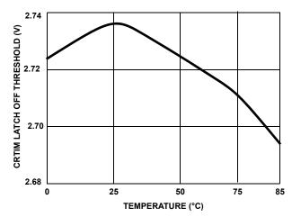
FIGURE 13. CRTIM THRESHOLD VOLTAGE vs TEMPERATURE
