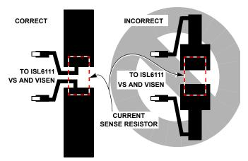
FIGURE 2. SENSE RESISTOR PCB LAYOUT
