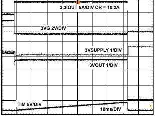
FIGURE 18. 3.3V INTO CR (VCRSET = 0.461V)
