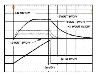
FIGURE 15. ISL6111 TURN-ON INTO M12V OC CONDITION
