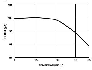
FIGURE 12. CRSET CURRENT vs TEMPERATURE
