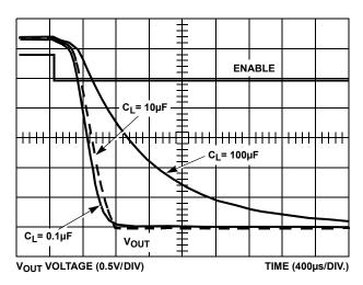
FIGURE 8. SLOW TURN-OFF vs  $C_{L}$ ,  $R_I = 8\Omega$
