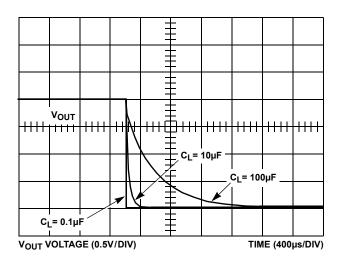
FIGURE 9. FAST TURN-OFF vs C<sub>LOAD</sub>
