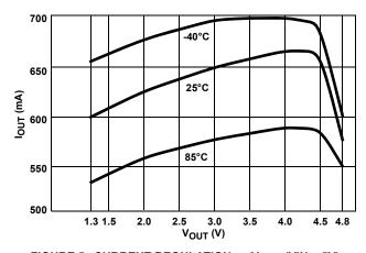
FIGURE 5. CURRENT REGULATION vs V<sub>OUT</sub> (VIN = 5V)
