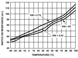
FIGURE 2. SWITCH ON RESISTANCE AT 0.4A
