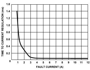
FIGURE 7. CR SETTLING TIME vs FAULT CURRENT
