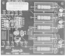
FIGURE 14. ISL6118EVAL1 SCHEMATIC AND PHOTOGRAPH
