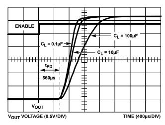
FIGURE 3.  $\text{V}_{\text{OUT}}$  SOFT START vs C  $_L$  and PROP DELAY,  $\text{R}_{\text{I}}$  = 8 $\Omega$
