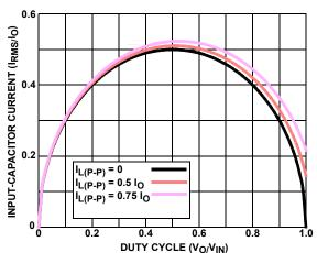
FIGURE 21. NORMALIZED INPUT-CAPACITOR RMS
