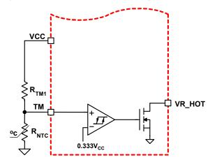
FIGURE 12. BLOCK DIAGRAM OF THERMAL MONITORING FUNCTION
