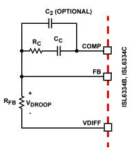
FIGURE 17. COMPENSATION CONFIGURATION FOR LOAD-LINE REGULATED ISL6334B, ISL6334C CIRCUIT
