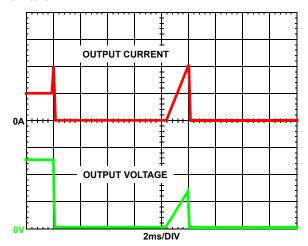
FIGURE 11. OVERCURRENT BEHAVIOR IN HICCUP MODE.  $F_{SW} = 500 \text{kHz}$
