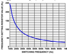
FIGURE 3. SWITCHING FREQUENCY vs RT
