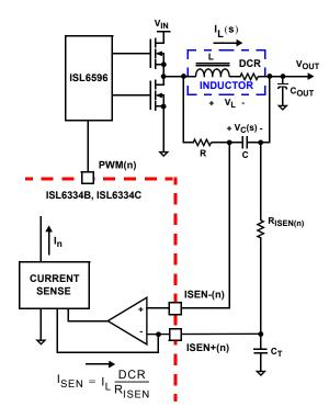
FIGURE 4. DCR SENSING CONFIGURATION
