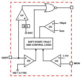
FIGURE 10. VR\_RDY AND PROTECTION CIRCUITRY
