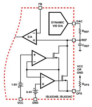
FIGURE 7. OUTPUT VOLTAGE OFFSET PROGRAMMING
