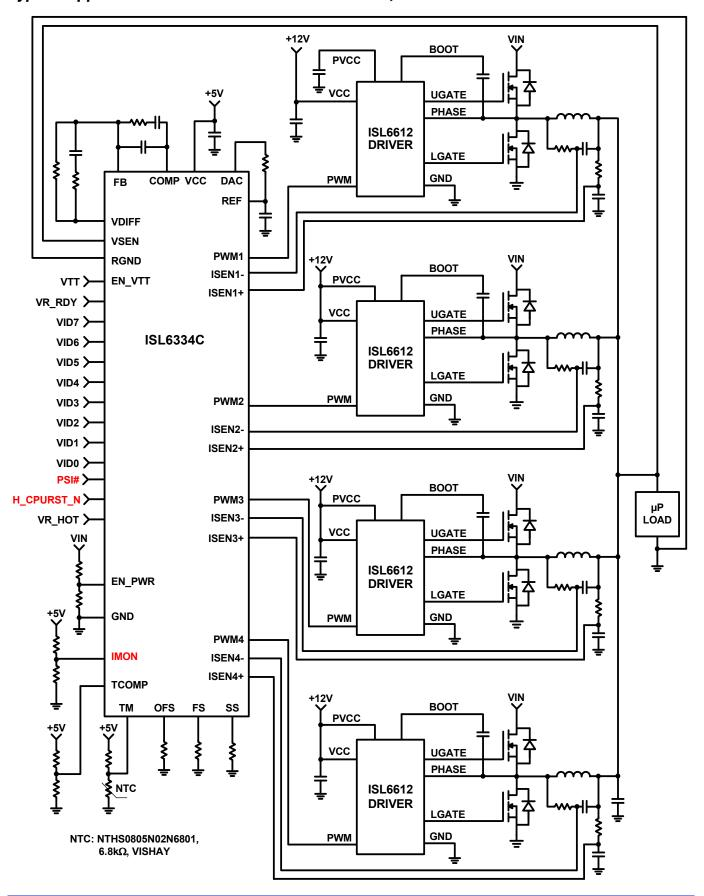
Typical Application - CI VR with External Thermal Compensation, 2-Phase PSI# (no DE and GVOT)
