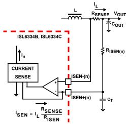
FIGURE 5. SENSE RESISTOR IN SERIES WITH INDUCTORS
