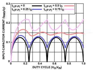
FIGURE 20. NORMALIZED INPUT-CAPACITOR RMS CURRENT VS DUTY CYCLE FOR 4-PHASE CONVERTER
