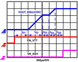
FIGURE 9. SOFT-START WAVEFORMS
