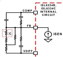
FIGURE 16. EXTERNAL TEMPERATURE COMPENSATION
