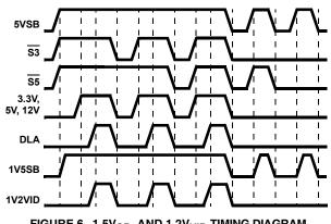
FIGURE 6. 1.5V<sub>SB</sub>, AND 1.2V<sub>VID</sub> TIMING DIAGRAM
