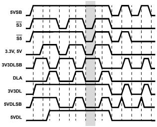
FIGURE 5. 5V<sub>DUAL</sub> AND 3.3V<sub>DUAL</sub>/3.3V<sub>SB</sub> TIMING DIAGRAM; ISL6504A
