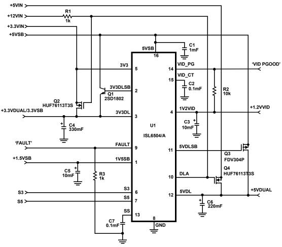
FIGURE 12. TYPICAL ISL6504/A APPLICATION DIAGRAM
