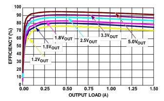
FIGURE 3. EFFICIENCY vs LOAD,  $V_{IN} = 7V$
