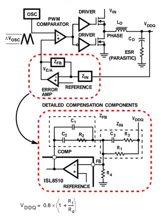
FIGURE 30. VOLTAGE-MODE BUCK CONVERTER
