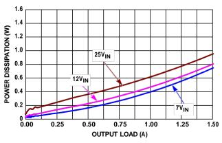
FIGURE 12. POWER DISSIPATION vs LOAD, 3.3VOUT
