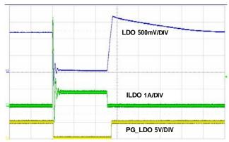
FIGURE 28. LDO SHORT CIRCUIT AND RECOVERY, 200µs/DIV
