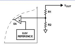
FIGURE 29. EXTERNAL RESISTOR DIVIDER
