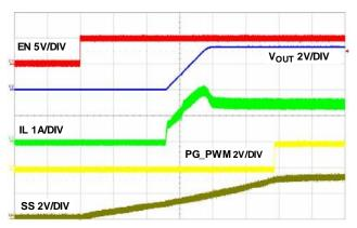
FIGURE 22. SOFT-START AT FULL LOAD, 500µs/DIV
