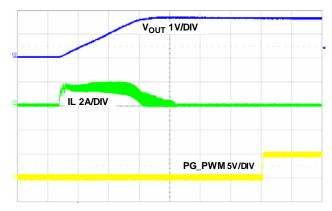
FIGURE 27. OUTPUT SHORT CIRCUIT RECOVERY, 200µs/DIV
