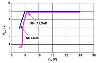
FIGURE 16.  $V_{CC}$  REGULATION WITH  $V_{IN}$
