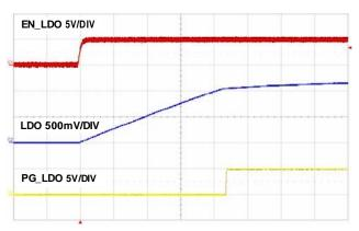
FIGURE 23. SOFT-START AT FULL LOAD, 100µs/DIV
