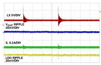
FIGURE 18. STEADY STATE OPERATION AT NO LOAD,  $20\mu\text{s}/\text{DIV}$
