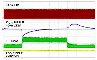
FIGURE 20. LOAD TRANSIENT, 200µs/DIV
