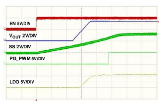
FIGURE 21. SOFT-START AT NO LOAD, 500µs/DIV
