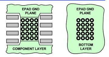
FIGURE 18. TYPICAL PCB PATTERN FOR THERMAL VIAS
