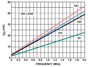
FIGURE 12. I<sub>DD</sub> vs FREQUENCY (+25°C)
