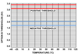
FIGURE 2. TEMPERATURE STABLE LOGIC THRESHOLDS
