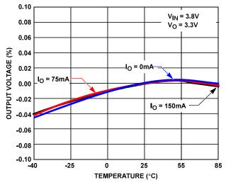
FIGURE 4. OUTPUT VOLTAGE vs TEMPERATURE
