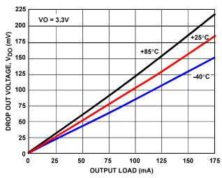
FIGURE 8. DROPOUT VOLTAGE vs LOAD CURRENT
