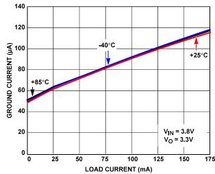
FIGURE 10. GROUND CURRENT vs LOAD
