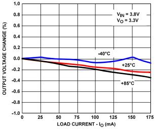
FIGURE 3. OUTPUT VOLTAGE vs LOAD CURRENT
