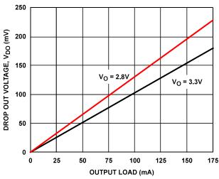
FIGURE 7. DROPOUT VOLTAGE vs LOAD CURRENT
