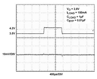
FIGURE 14. LINE TRANSIENT RESPONSE, 2.8V OUTPUT
