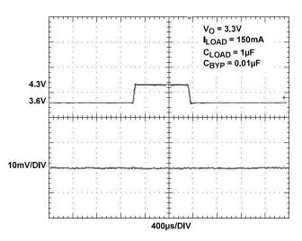
FIGURE 13. LINE TRANSIENT RESPONSE, 3.3V OUTPUT
