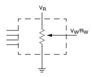
Three terminal Potentiometer; Variable voltage divider
