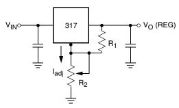
$V_{O}(REG) = 1.25V (1+R_2/R_1)+I_{adj} R_2$
