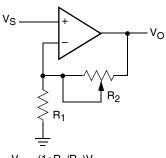
$V_0 = (1 + R_2/R_1)V_S$
