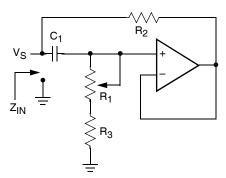
$$\begin{split} Z_{IN} = R_2 + s \; R_2 \; (R_1 + R_3) \; C_1 = R_2 + s \; \text{Leq} \\ (R_1 + R_3) >> R_2 \end{split}$$
