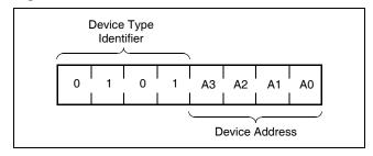
The next four bits of the slave address are the device address. The physical device address is defined by the state of the  $A_0$  -  $A_3$  inputs. The X9418 compares the serial data stream with the address input state; a successful compare of all four address bits is required for the X9418 to respond with an acknowledge. The  $A_0$  -  $A_3$  inputs can be actively driven by CMOS input signals or tied to  $V_{CC}$  or  $V_{SS}$ .
