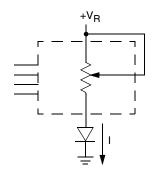
Two terminal Variable Resistor; Variable current
