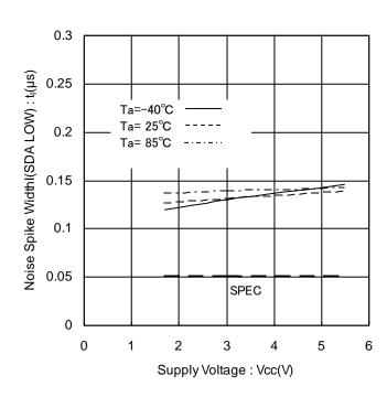
Figure 31. Noise Spike Width vs Supply Voltage (SDA LOW)
