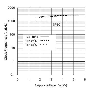
Figure 13. Clock Frequency vs Supply Voltage
