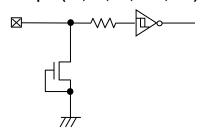
Figure 50. Input Pin Circuit Diagram
