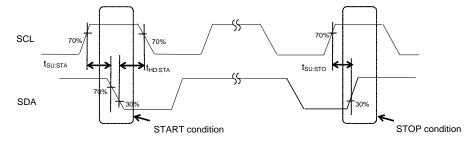
Figure 2-(b). Start-Stop Bit Timing
