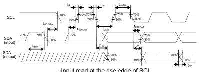
olnput read at the rise edge of SCL oData output in sync with the fall of SCL Figure 2-(a). Serial Input / Output Timing
