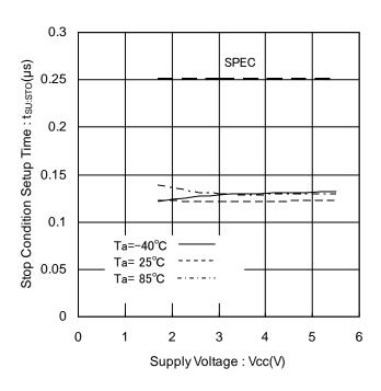
Figure 25. Stop Condition Setup Time vs Supply Voltage
