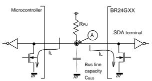
Figure 45. I/O Circuit Diagram
