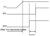
Figure 53. When SCL= 'H' and SDA= 'L' Figure 54. When SCL='L' and SDA='L'
