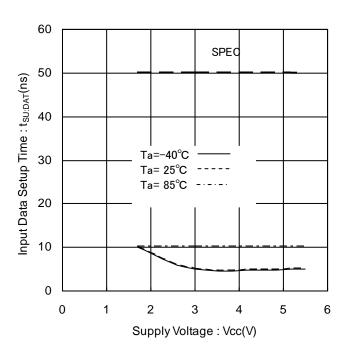
Figure 22. Input Data Setup Time vs Supply Voltage (LOW)
