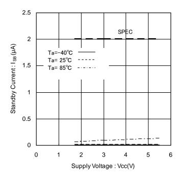
Figure 12. Standby Current vs Supply Voltage
