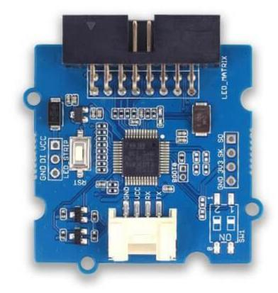
Grove - LED Matrix Driver v1.0 is UART (Serial) to dot matrix LED driver that incorporates various graphics functions. It can only support 32×64 LED matrix. This product is a **Grove** compatible UART interface. It provides easy and rich APIs that abstract the complexity of the underlying LED driving hardware. All you need to is just call these APIs in code to implement different functionalities for your project.
