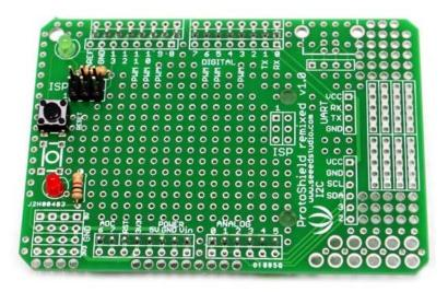
**Step 2:** Solder the female and male connectors. Note: solder ADC6 and ADC7 **ONLY** if your are using a Seeeduino. When using an Arduino, do **NOT** solder ADC6 and ADC7.
