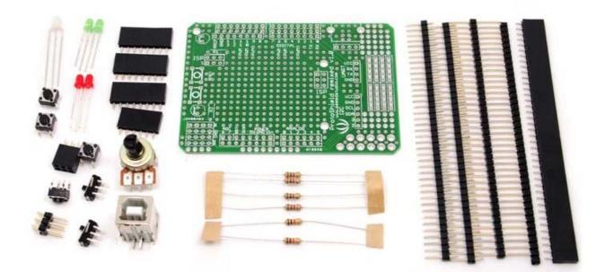
Build your own Arduino shield using the compact and flexible Proto Shield kit. Solder together a limitless range of circuits and reuse it in all your Arduino projects. A standard 0.1" prototyping grid accepts commonly used through-hole parts and chips. Basic components (resistors, potentiometer, LEDs, switches) are included to help you get started with your custom shield.
