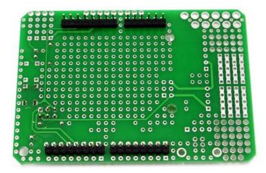
**Step 3:** Solder the USB connector to the USB port, and the potentiometer in the 80 mil holes. Solder the bottom left Power pins to suit your project.
