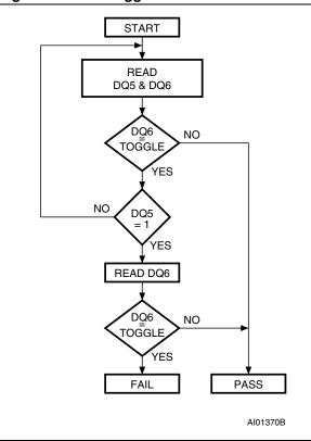
The Error Flag (DQ5) bit is set if either an internal time-out occurred while the embedded algorithm attempted to program the byte, or if the DSP attempted to program a 1 to a bit that was not erased (not erased is logic 0).
