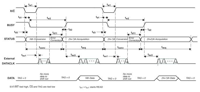
Figure 3. Basic Conversion Timing (External DATACLK)
