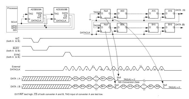
Figure 27. Timing of TAG Feature With Single Conversion (Using External DATACLK)
