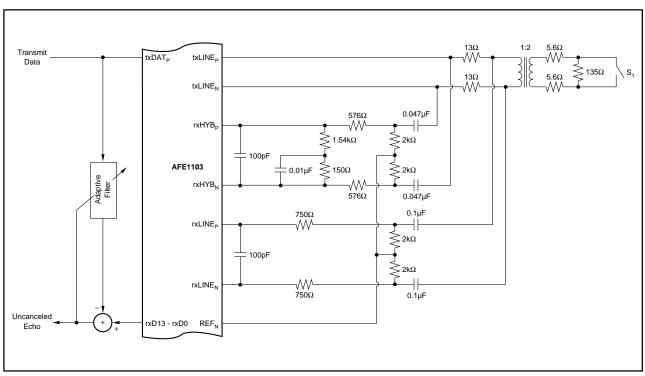
FIGURE 4. Uncancelled Echo Test Diagram.
