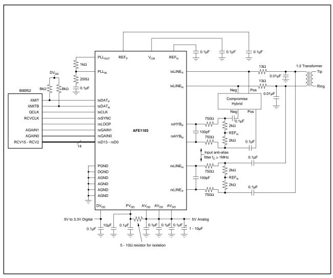
FIGURE 2. Basic Connection Diagram.
