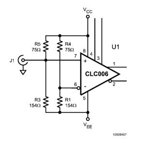
FIGURE 4. Single Ended  $50\Omega$  ECL input
