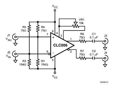
FIGURE 9. Differential Input Reduced Output
