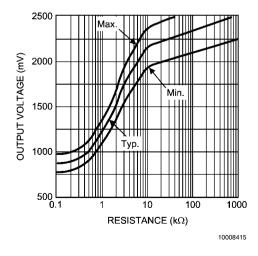
FIGURE 12. Resistance Pins 3 to 4 vs Output Voltage Increased Output @  $150\Omega$  Load
