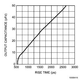
FIGURE 13. Rise Time vs C<sub>L</sub>
