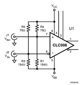
FIGURE 5. Differential  $50\Omega$  ECL Input
