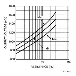
FIGURE 10. Resistance Pins 3 to 4 vs Output Voltage Reduced Output @  $150\Omega$  Load
