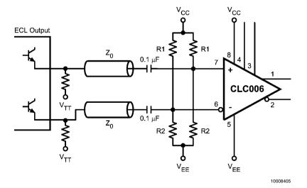
FIGURE 2. AC Coupled Input
