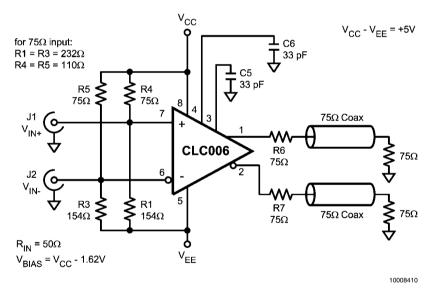
FIGURE 7. Differential Input DC Coupled Output
