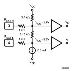
FIGURE 8. Equivalent Bias Generation Circuit
