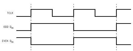
Figure 4. "Worst Case" Serializer ICC Test Pattern
