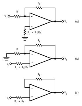
Figure 54. Canceling the Voltage Offset Effect of Input Bias Current
