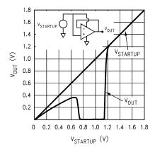
Figure 55. Output Voltage vs. Supply Voltage
