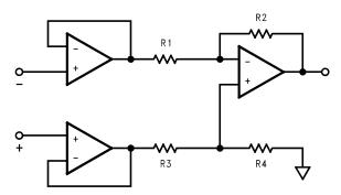
Figure 58. Rail-to-rail instrumentation amplifier
