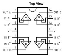
Figure 61. 14-Pin TSSOP/SOIC **Package**
