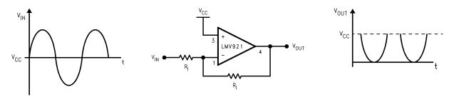
Figure 57. Half-Wave Rectifier with Negative-Going Output Referenced to V<sub>CC</sub>
