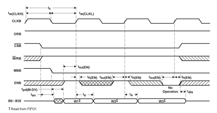
Figure 5. Port-B Read-Cycle Timing for FIFO1
