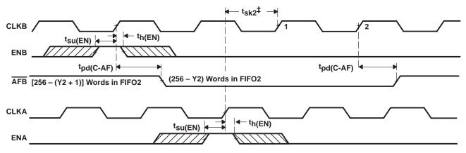
‡t<sub>sk2</sub> is the minimum time between a rising CLKB edge and a rising CLKA edge for AFB to transition high in the next CLKB cycle. If the time between the rising CLKB edge and rising CLKA edge is less than  $t_{sk2}$ ,  $\overline{AFB}$  may transition high one CLKA cycle later than shown. NOTE A: FIFO2 write (CSB = L, W/RB = L, MBB = L), FIFO2 read (CSA = L, W/RA = L, MBA = L). Data in the FIFO2 output register has been read from the FIFO.
