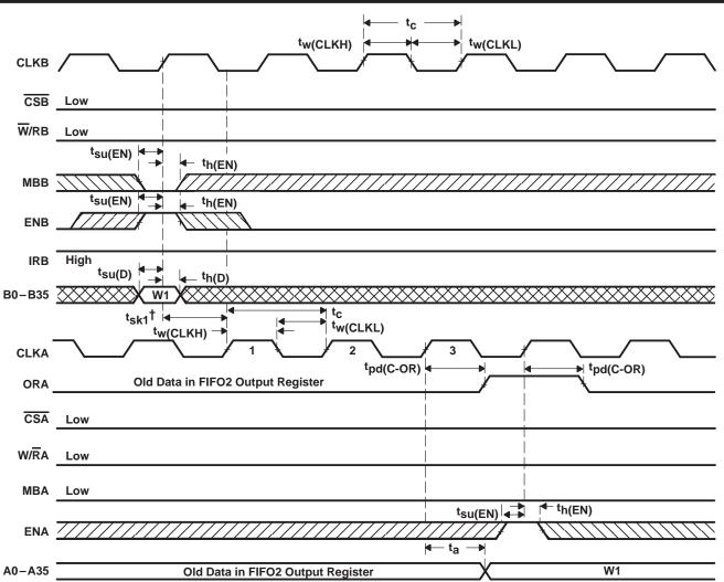
t tsk1 is the minimum time between a rising CLKB edge and a rising CLKA edge for ORA to transition high and to clock the next word to the FIFO2 output register in three CLKA cycles. If the time between the rising CLKB edge and rising CLKA edge is less than tsk1, the transition of ORA high and load of the first word to the output register may occur one CLKA cycle later than shown.
