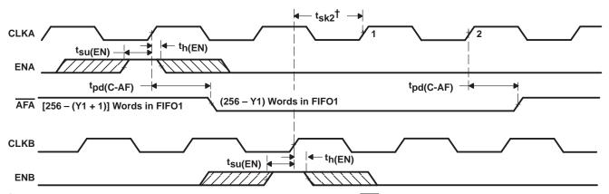
t sk2 is the minimum time between a rising CLKA edge and a rising CLKB edge for AFA to transition high in the next CLKA cycle. If the time between the rising CLKA edge and rising CLKB edge is less than t<sub>sk2</sub>, AFA may transition high one CLKB cycle later than shown. NOTE A: FIFO1 write (CSA = L, W/RA = H, MBA = L), FIFO1 read (CSB = L, W/RB = H, MBB = L). Data in the FIFO1 output register has been read from the FIFO.
