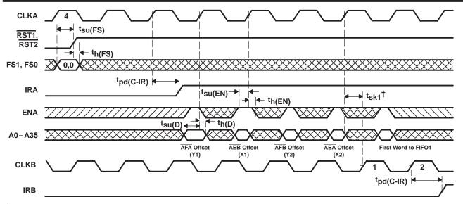
tsk1 is the minimum time between the rising CLKA edge and a rising CLKB edge for IRB to transition high in the next cycle. If the time between the rising edge of CLKA and rising edge of CLKB is less than t<sub>sk1</sub>, IRB may transition high one cycle later than shown. NOTE A: CSA = L, W/RA = H, MBA = L. It is not necessary to program offset register on consecutive clock cycles.
