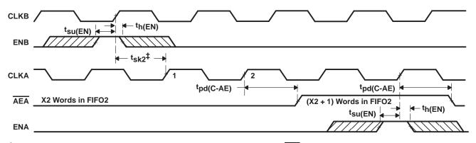
t<sub>sk2</sub> is the minimum time between a rising CLKB edge and a rising CLKA edge for AEA to transition high in the next CLKA cycle. If the time between the rising CLKB edge and rising CLKA edge is less than t<sub>sk2</sub>, AEA may transition high one CLKA cycle later than shown.
