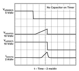
Figure 7. Channel 2 Overcurrent Response:
