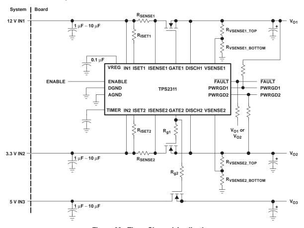
Figure 28. Three-Channel Application
