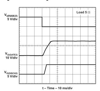
Figure 3. Turnon Voltage Transition of Channel 2
