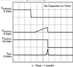
Figure 10. Channel 2 - Enabled Into Short Circuit
