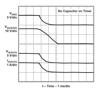
Figure 14. Channel 2 - Hot Removal
