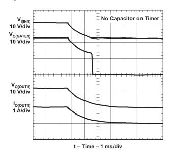
Figure 12. Channel 1 - Hot Removal
