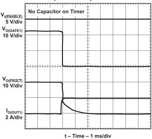
Figure 6. Channel 1 Overcurrent Response: an Overcurrent
