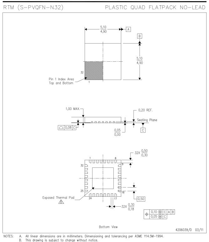
С. Д QFN (Quad Flatpack No-Lead) Package configuration.
