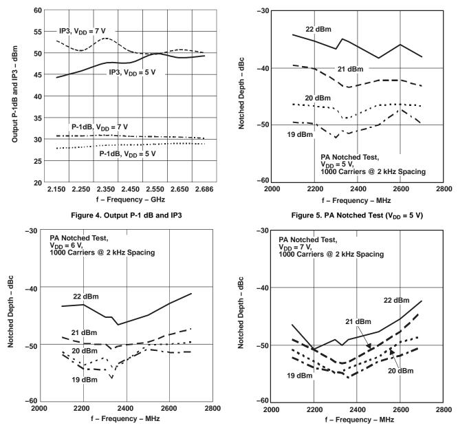
Figure 6. PA Notched Test (V<sub>DD</sub> = 6 V)
