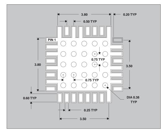
SOLDER MASK: NO SOLDERMASK UNDER CHIP, ON LEAD PADS OR ON GROUND CONNECTIONS. 25 VIA HOLES, EACH 0.38 mm. DIMENSIONS in mm
