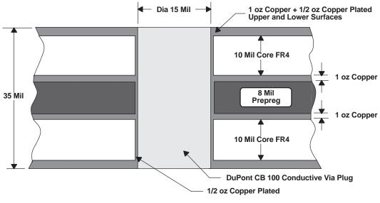
Figure 12. PCB Via Cross Section
