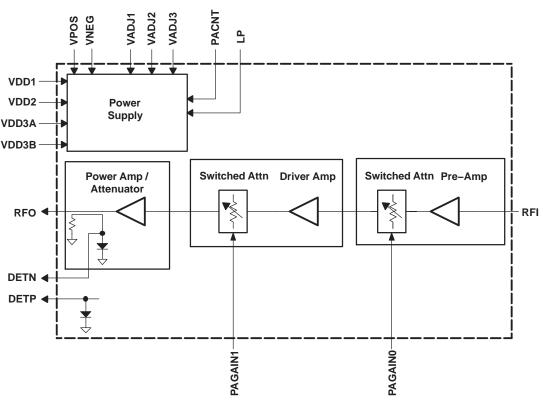
Figure 1. Detailed Block Diagram of TRF1123
