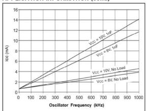
Figure 8. UCC3813-0 I<sub>CC</sub> vs. oscillator frequency.
