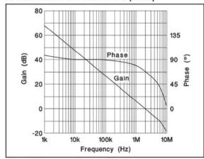
Figure 2. Error amplifier gain/phase response.
