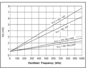
Figure 10. UCC3813-5 I<sub>CC</sub> vs. oscillator frequency.
