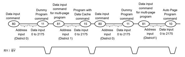
After either "15h" or "10h" Program command is input to the device, physical programing starts as follows. For details about Auto Page Program with Data Cache, refer to "Auto Page Program Operation with Data Cache".
