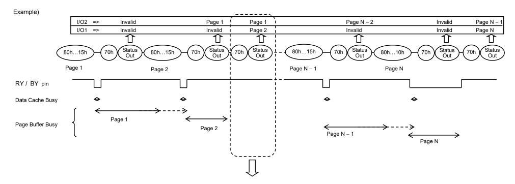
If the Page Buffer Busy returns to Ready before the next 80h command input and Status Read is done during this Ready period, the Status Read provides the Pass/Fail result for Page 2 on I/O1 and the Pass/Fail result for Page1 on
