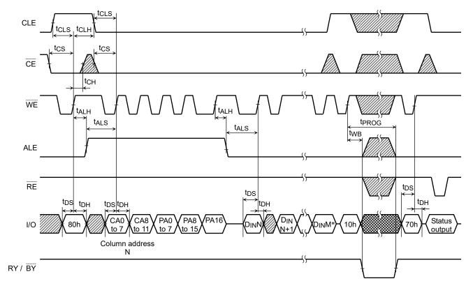
: Do not input data while data is being output.
