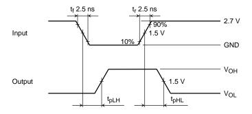
Figure 2 t<sub>pLH</sub>, t<sub>pHL</sub>
