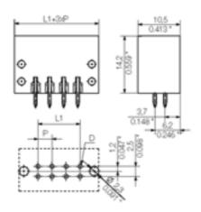
Order No. 1729590000 S2L 3.5/6/180F3.5SN SW Part designation Version PCB plug-in connector, Male connectors, Soldered
