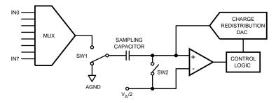
Figure 35. ADC088S022 in Hold Mode
