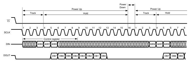
Figure 1. ADC088S022 Operational Timing Diagram
