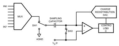
Figure 34. ADC088S022 in Track Mode
