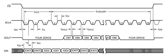
Figure 2. ADC088S022 Serial Timing Diagram
