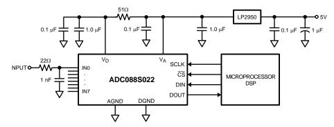
Figure 38. Typical Application Circuit
